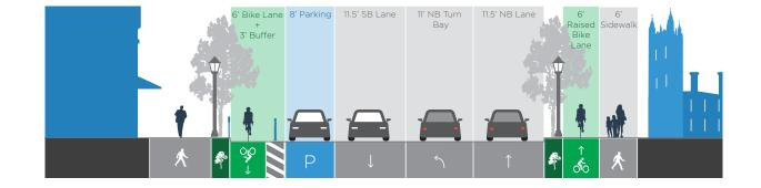
At the Nassau Presbyterian Church, northbound bicyclists are transitioned on-road to a one-way separated bike lane. The existing taxi stand would be relocated to another area. Parking is removed from the southbound side, and the southbound one-way separated bicycle lane continues along the curb.
