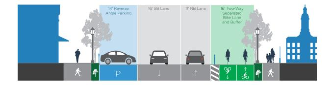
Approaching the Washington Road intersection, an additional travel lane is provided in the northbound direction for turning vehicles. To accommodate the additional lane, the width of the southbound lane and the width of the two-way separated bike lane and buffer are reduced.
