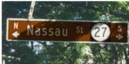
Street signs on traffic signals should have a brown background with white lettering.
