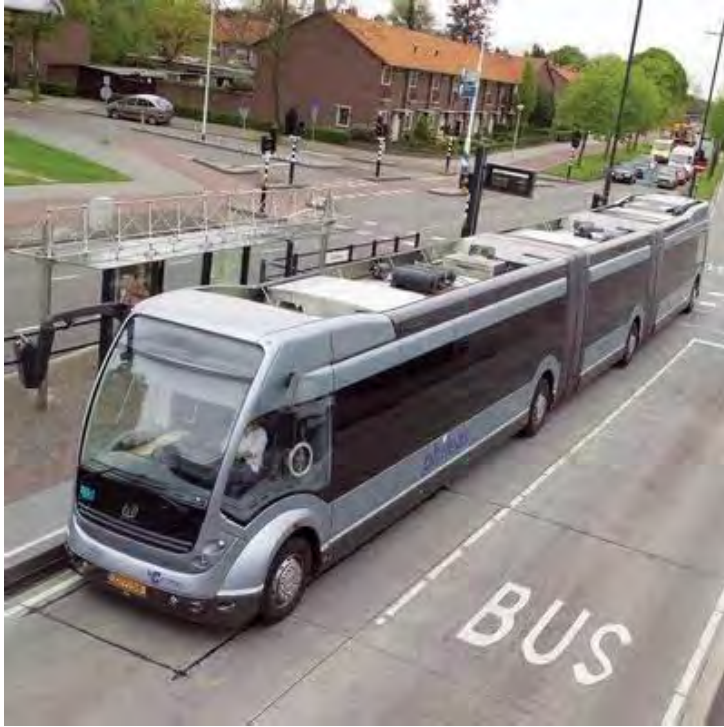
Figure 1-9. Phileas Magnetic guidance bus
