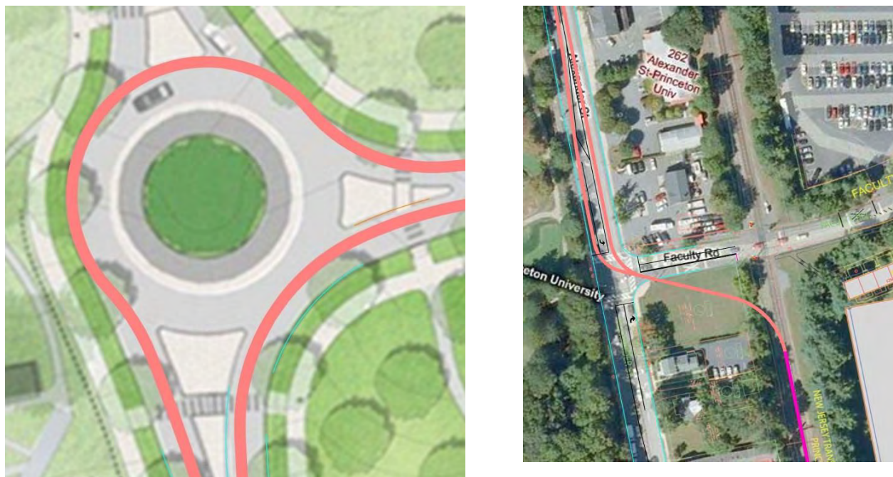
Figure 10: Streetcar alignment options through the Roundabout on left; on right, connection from Dinky line to Alexander Road in proximity of Faculty Road.
