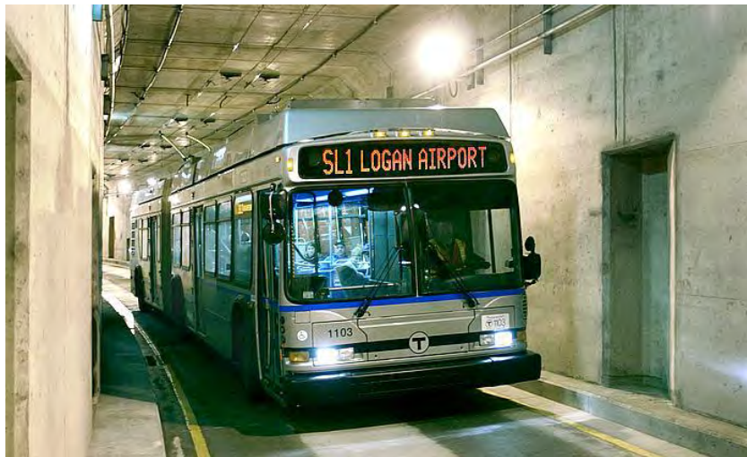
Figure 1-7 MBTA's Silver Line Operating on Dual Power Diesel/Electric
