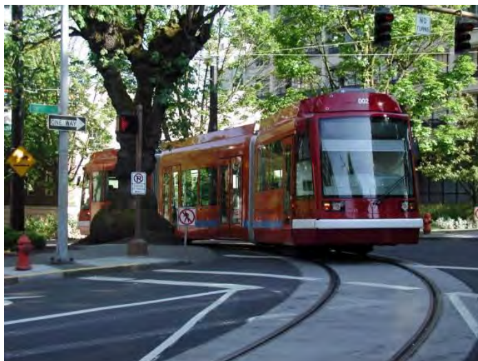
Figure 1-13 Skoda Streetcar in service in Portland Oregon utilizes overhead contact system
